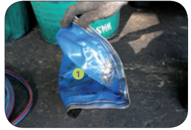
1 Damaged drum cover due to impact of the explosion
