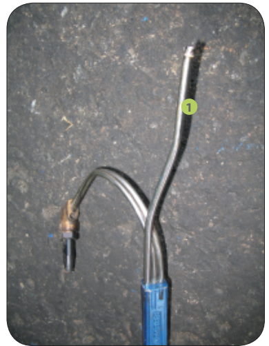
1 Damaged cutting torch due to impact of the explosion
