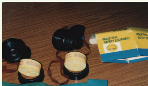
Incorrect respirators that do not protect against acid mists were used by the worker
